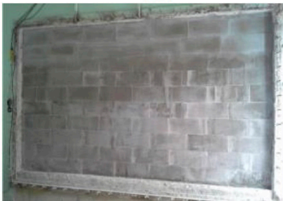
Tested wall with gypsum mortar
